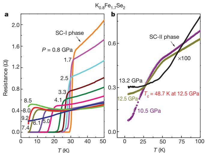
**Figure 3 | Temperature dependence of the resistance for  $\text{K}_{0.8}\text{Fe}_{1.7}\text{Se}_2$  at different pressures.** **a**, SC-I. The resistance–temperature curves showing the  $T_c$  reduction with increasing pressure and its disappearance at 9.2 GPa. **b**, SC-II. The resistance measurements reveal another superconducting phase above 10.5 GPa. The  $T_c$  reaches 48.7 K at 12.5 GPa and disappears at 13.2 GPa. The black curve has been multiplied by 100.
